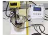
Water saturation determination with WSTM 01 set
