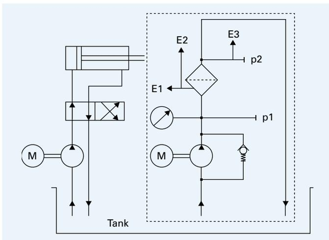
During off-line filtration, the filter operates in a cycle that is separate from the main system. By separating the systems, off-line filtration can take place independently of the system's running time until the desired fluid cleanliness is reached.
